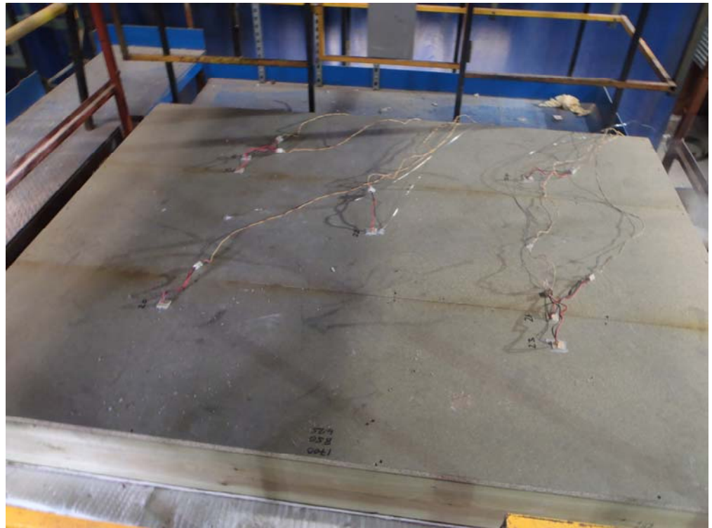
The unexposed face of the ceiling after a test duration of 60 minutes
