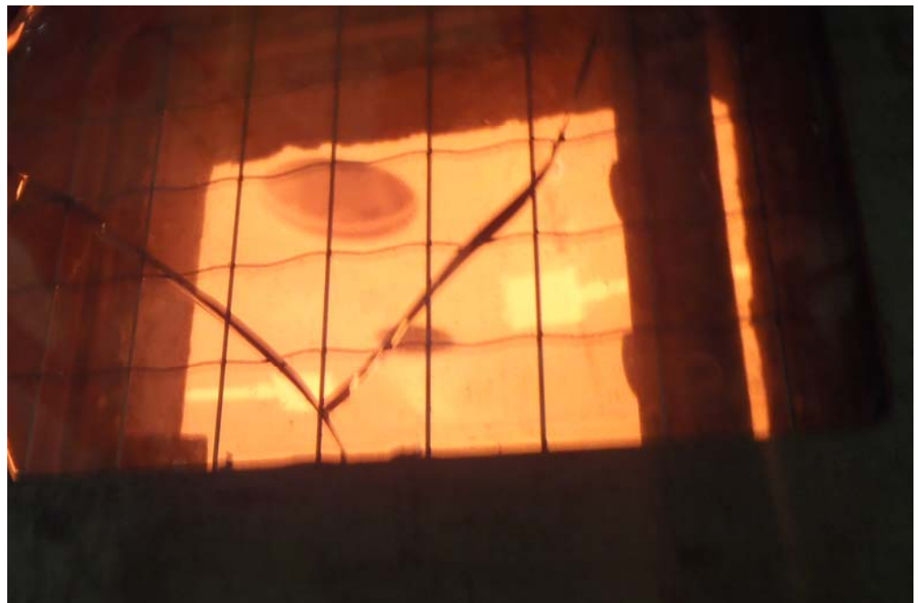
The exposed face of the ceiling after a test duration of 60 minutes
