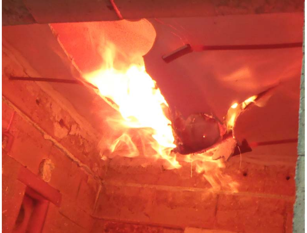
The exposed face of the ceiling immediately after the test
